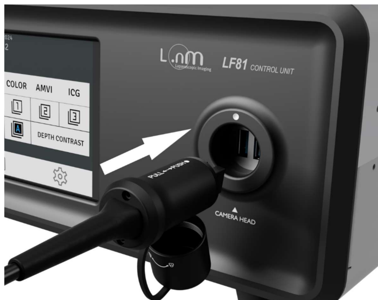
Fig 6.2: Camera Probe to CCU Connection
